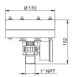
Vacuum regulator with flanged inlet connection
