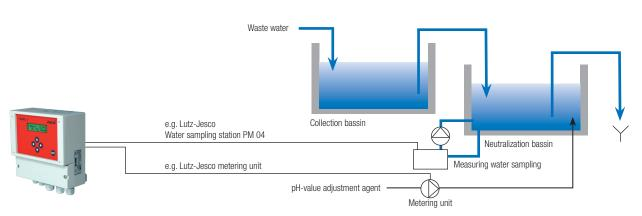
Records the actual pH-value of waste water before discharge into public sewerage system and controls the dosing of pH-value adjustment agent.
