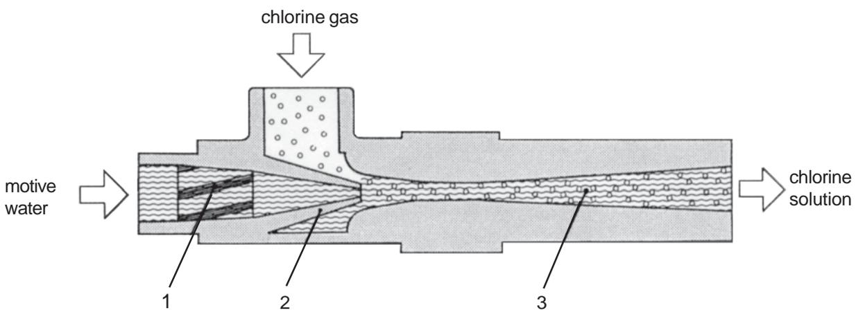
However, this very simple physical process presupposes that the motive pressure, backpressure and suction pressure are all correct. If they are not, the ejector may be unable to prime chlorine gas or cannot restart when switched off or simply cannot extract the required volume of chlorine gas.
