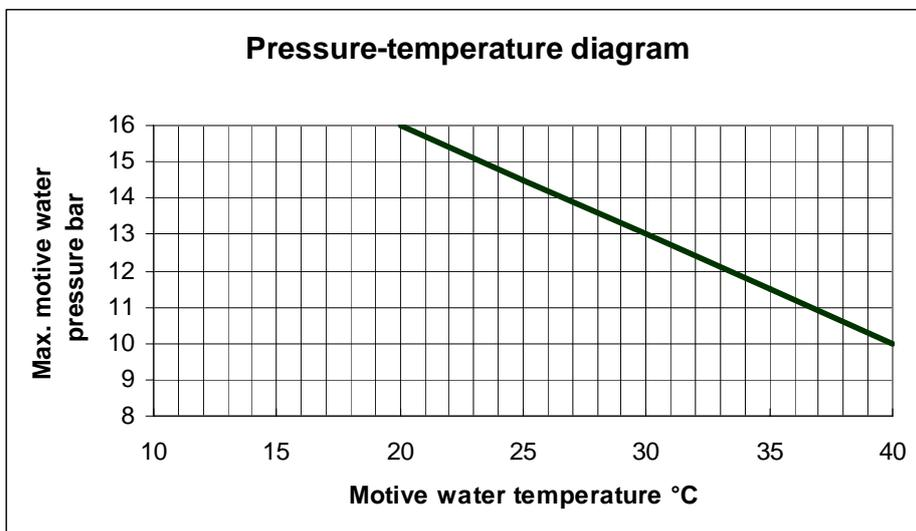
Injectors can be selected on the basis of the following parameters and corresponding working curves, with due regard for the motive water temperature (max. 40 °C).
