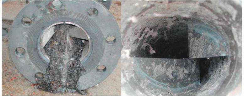
Typical clogging of competitor's mixer after less than 5 hours
